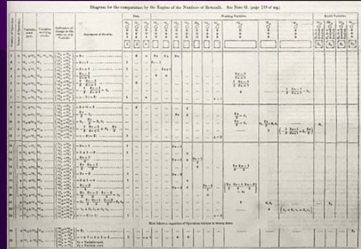
Lovelace's diagram from Note G, the first published computer algorithm
